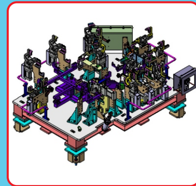
SPOT WELDING FIXTURE FOR DOOR INNER ASSY
